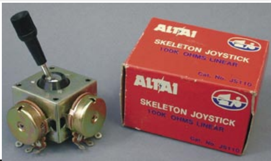
Figure 3 - Altai skeleton joystick
